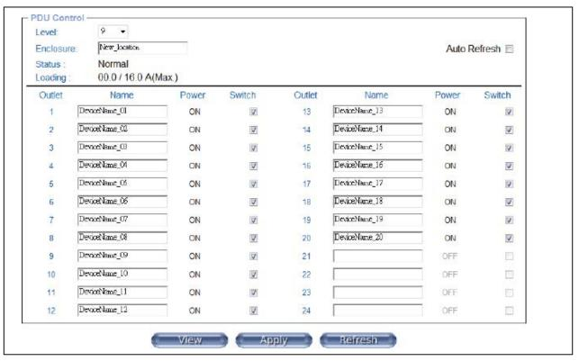
: show the specified PDU status (Select the PDU Level > View)
