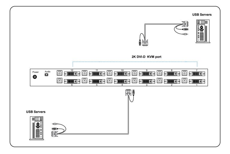
DVI KVM Cable CI - 6 : 6 feet DVI KVM cable CI - 15 : 15 feet DVI KVM cable ( Server end : DVI-D + USB + Audio ) ( KVM port : DVI-D + USB3.0 )
