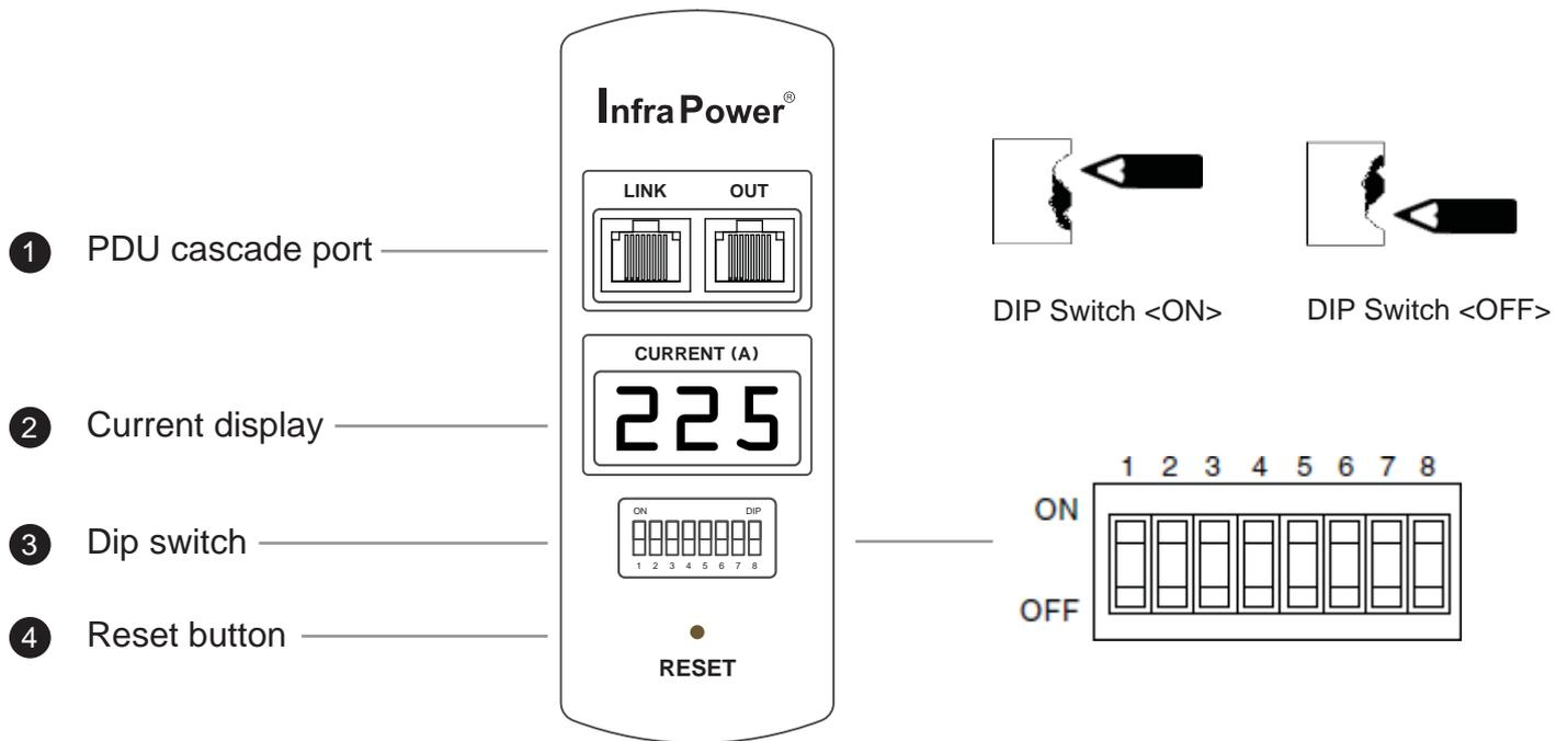
■ For rackmount PDU, ② ③ ④ on the front panel left , ① on the rear panel
