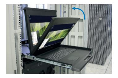
■ Flip up the LCD to a suitable angle.
