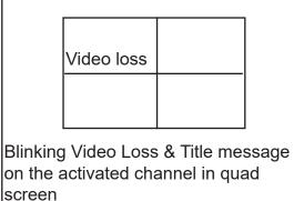
■ The warning message and the buzzer can be cleared by pushing Lock button (#2) for more than 4 seconds if the device is operated under Security lock On mode, or pushing any button on the front panel if the device is operated under Security lock OFF mode.
