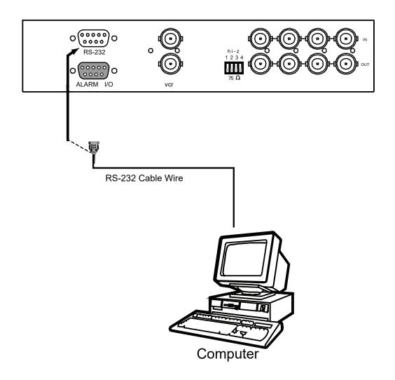
The device can be controlled via the male type 9 pin D-sub/RS-232 connector to a computer using ASCII code.
