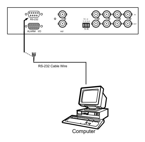
The device can be controlled via the male type 9 pin D-sub/RS-232 connector to a computer using ASCII code.
