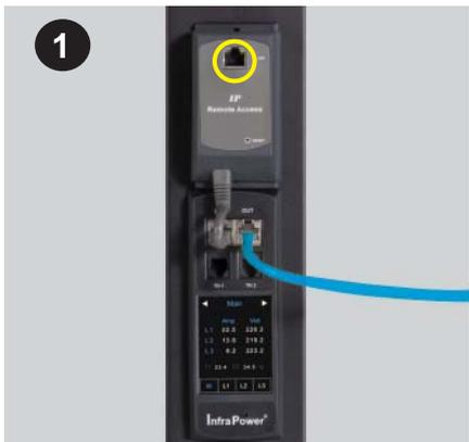
Step 1 - Disconnect LAN cable from the faulty IP dongle
