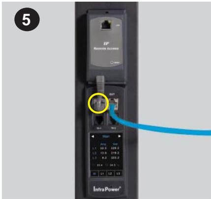
**Step 5 - Plug RJ-45 jack into the meter LINK port**
