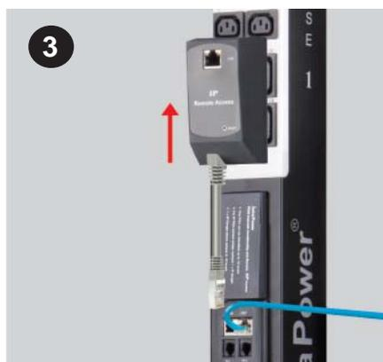
Step 3 - Slide out the faulty IP dongle from the plate
