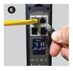
Step 6 - Reconnect LAN Cable & Sensor Cable
