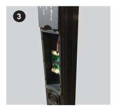
Step 3 - Unscrew and pull out the faulty W meter.
