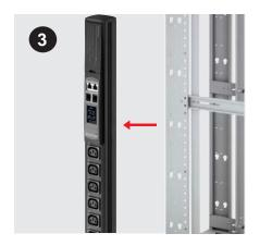
Step 3 - Take out the faulty PDU
