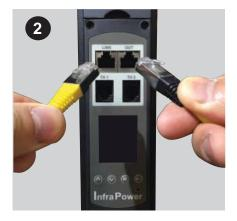
Step 2 - Disconnect LAN Cable & Sensor Cable - Power Down the PDU
