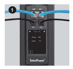
Step 1 - Mark down the PDU level no
