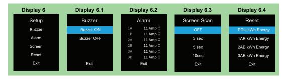
Step 1 - Press the 4 / button to Display 6 and press to confirm.
